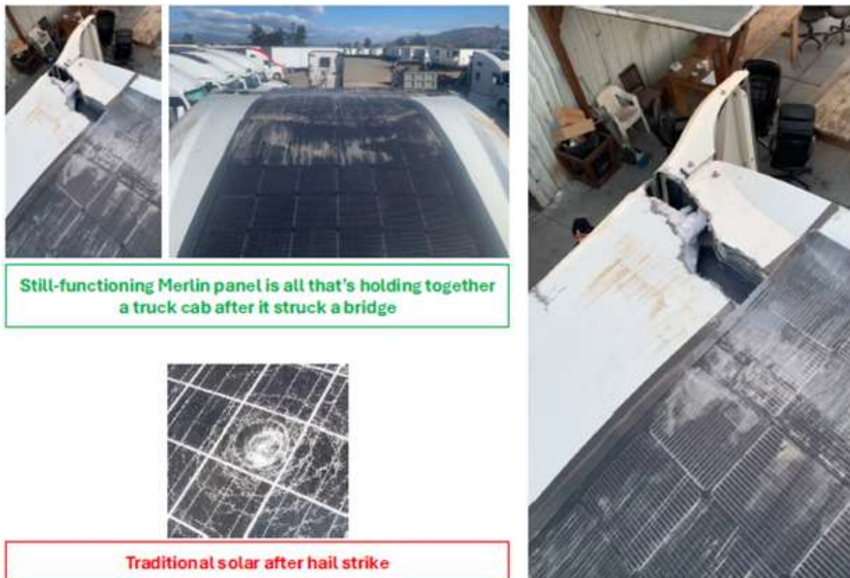
Figure 4.6. Field validation of mechanical durability following severe impact. A Merlin Solar flexible crystalline silicon module installed on a commercial truck cab fairing remained electrically functional and structurally intact after the vehicle struck an overbridge, resulting in significant damage to the surrounding fiberglass structure. The panel continued to generate power and contributed to stabilizing the damaged fairing. For comparison, conventional glass-framed photovoltaic modules subjected to similar impact or hail events typically exhibit cell fracture, glass breakage, and loss of electrical continuity at substantially lower mechanical loads.
