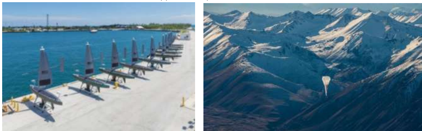
Figure 6.7. Several autonomous ocean drones equipped with Merlin Solar panels.
