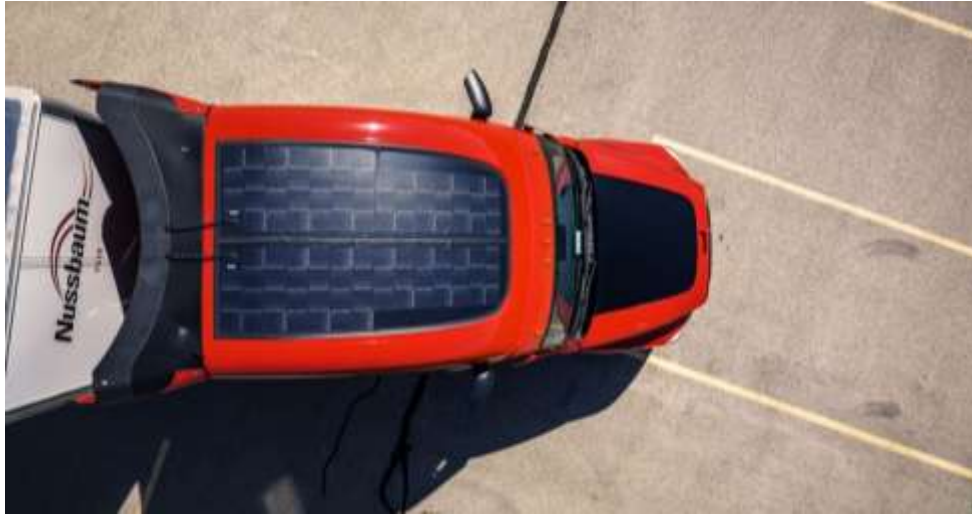
Figure 6.2. Merlin Solar direct-fit panels installed on a Freightliner Cascadia cab fairing.
