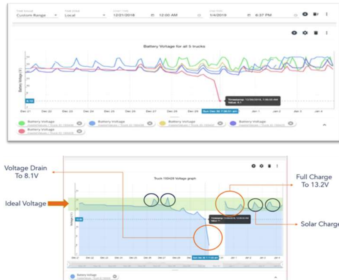
Figure 5.4. Field-recorded battery voltage traces from a multi-vehicle pilot deployment illustrating Merlin Solar’s ability to prevent deep-discharge events under extended auxiliary load conditions. (Top) Aggregate battery voltage profiles across multiple trucks over a multi-day period. (Bottom) Representative vehicle trace highlighting voltage stabilization above the deep-discharge threshold (~8.1 V) and recovery toward full charge levels (~13.2 V) enabled by continuous solar charging. Results demonstrate improved battery protection, reduced jump-start risk, and enhanced operational reliability.
