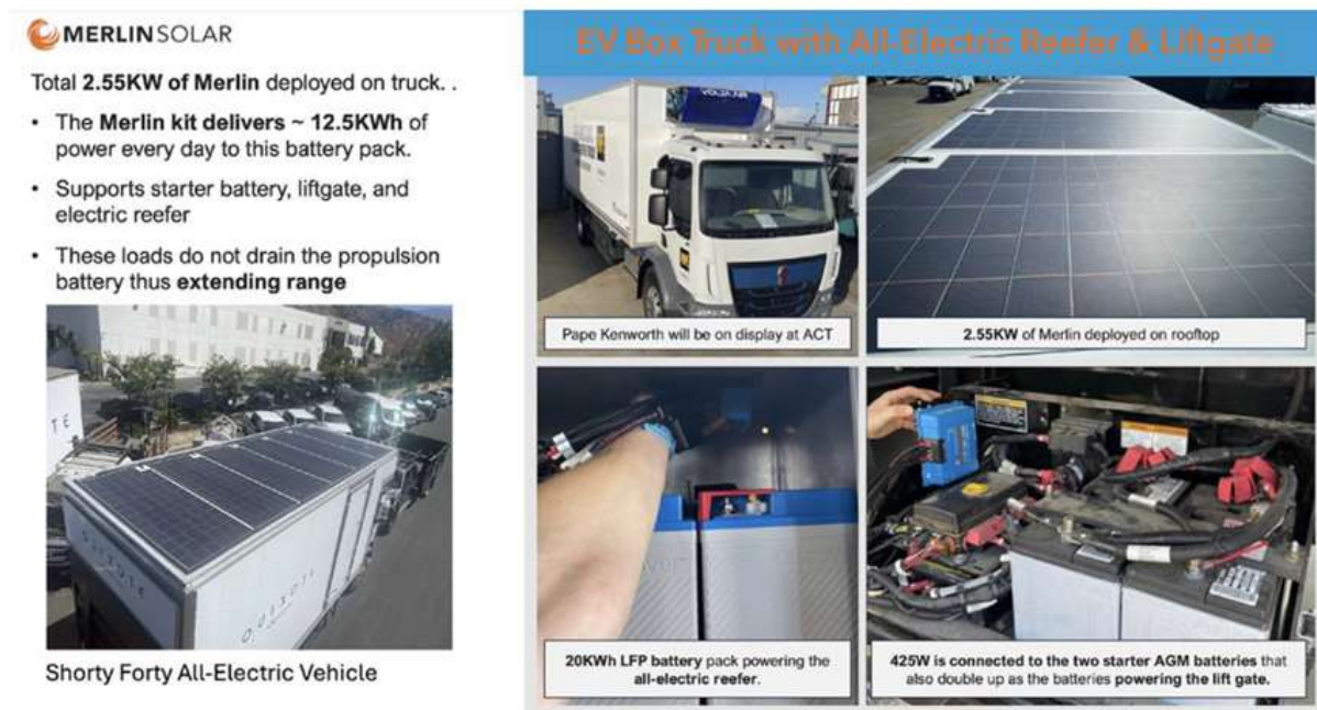
Figure 6.5. 2.55 kW Merlin Solar array integrated on the box truck roof, delivering daily solar energy to a 20 kWh LFP battery pack and AGM starter batteries to support refrigeration and liftgate loads independent of propulsion energy.
